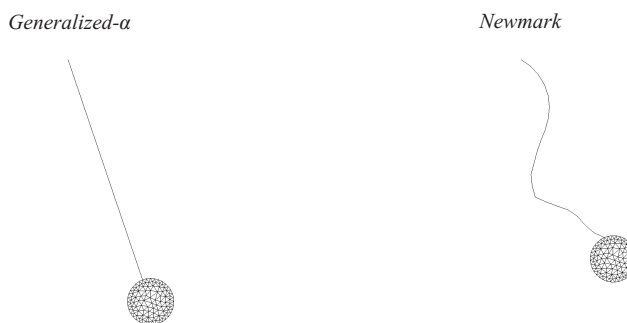
Figure 3.33 Deformed cable at time 2.78 s.
