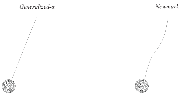
Figure 3.31 Deformed cable at time 2.18 s.
