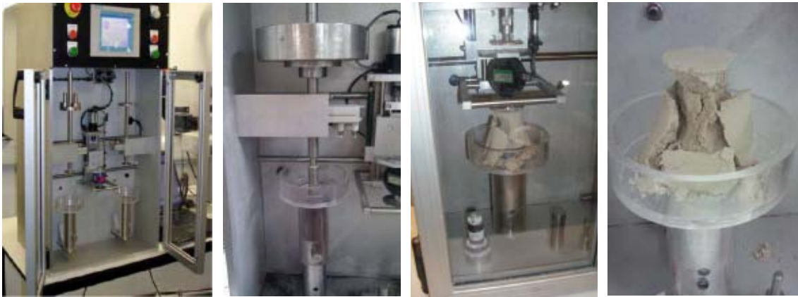
Figure 1 - (From left to right) Edinburgh Powder Tester (EPT), confined consolidation, unconfined compression and failed material sample
