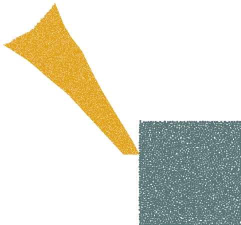
Figure 9.5: Initial set-up of 2D model of rock cutting with a ripper
