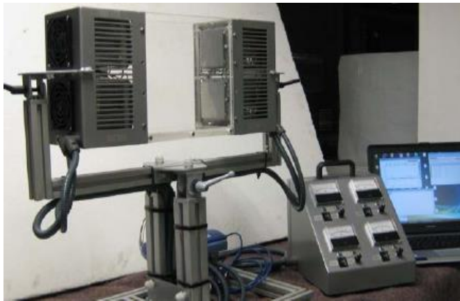
Figure 1. The Thermolectric Convective Didactive Device (TCDD) with its control panel, computer measuring and control of temperature.
