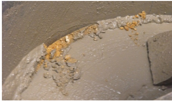
Figure 1: Example of an inadequate mixing, some dry constituents remain in the mixer
