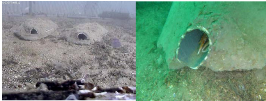
Figure 2.1.2. Images of the created enclosure in PVC material holding a contention net plus PVC tunnels embedded in concrete material, as deployed in front of the small satellite camera of the OBSEA platform. A frame depicting an animal in “door-keeping” behaviour ( sensu Aguzzi et al., 2007) is also reported.
