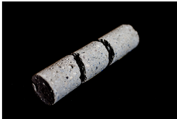
Figure 1: Concrete specimen, destroyed by spall fraction. (Photography: Ulrich van Stipriaan)
