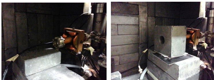
Figure 3. Left: view of the e-beam exit. Right: X-rays lead collimator in front of the e-beam exit.
