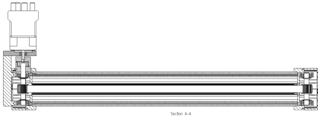
Figure 16: Section of the Y-axis mechanism
