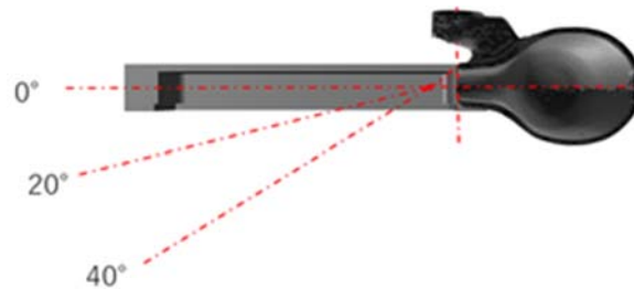
Fig.2 The angle between ladle and sleeve
