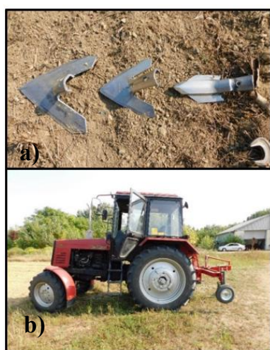
Figure 3: a) cultivator tools, the piece in the middle was used for tillage experiments b) the tractor
