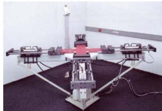
Figure 1: Biaxial testing machine of the Essener Labor für Leichte Flächentragwerke at the University of Duisburg-Essen with a maximum load of 50 kN in each direction
