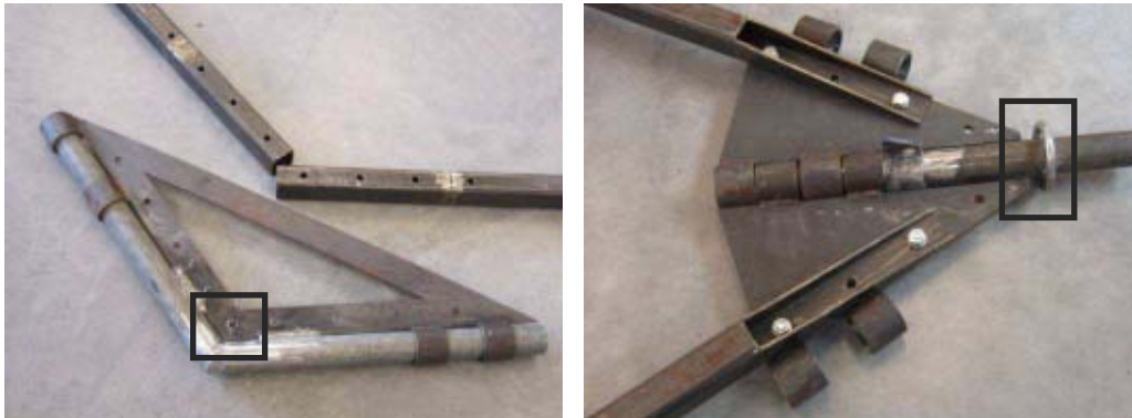
Figure 10. Modified connections: a. welded bars and an additional hole in the plate b. ring to attach the belts
