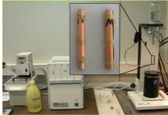
Figure 5: Dilatometer test with rolled specimens for determining of the CTE values
