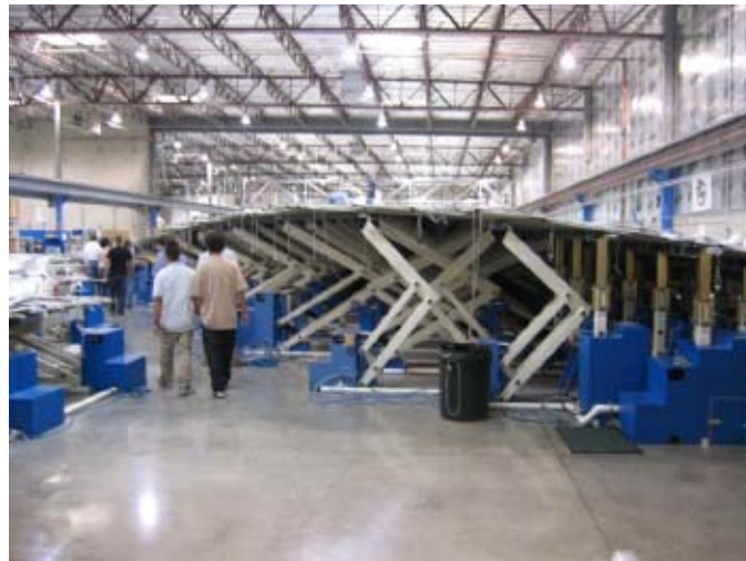
Figure 7: North Sails mould with numerous actuators.
