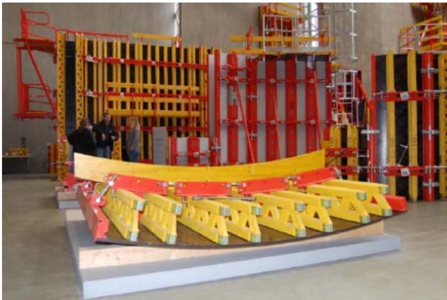
Figure 4: Photo showing PERI's single curvature scaffolding.
