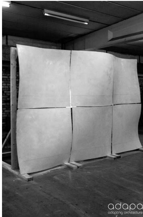
Figure 12: Surface made up of elements produced with the double sided mould technique.
