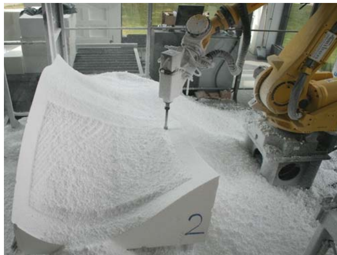
Figure 1: Photo of a robot CNC-machine milling in a styropor material.
