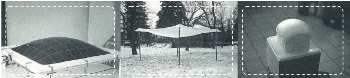
Figure 5: Isler's Experimental Forms, based on air pressure, gravity and material flow 5
