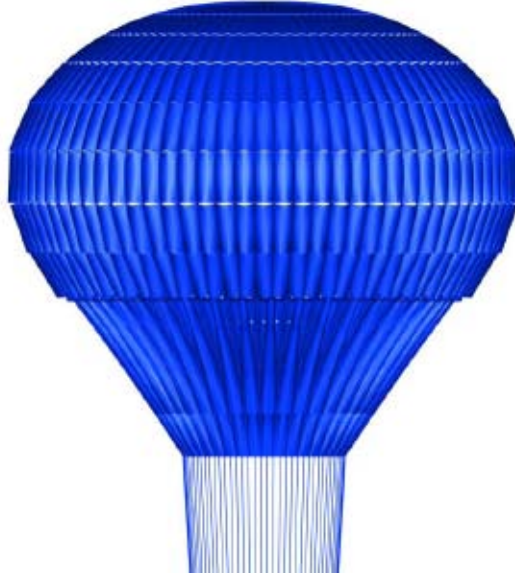
Figure 3: Structural mechanics solution for the parachute reefed to \tau_{REEF} = 13\% (approximately), obtained with the SCFSI M2C computation and the refined structure mesh.
