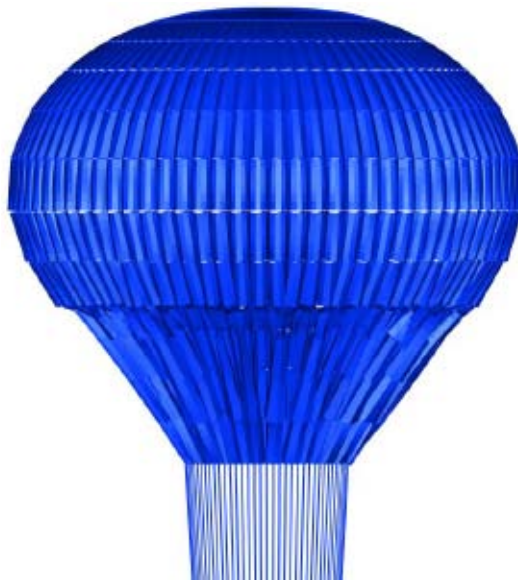
Figure 1: Structural mechanics solution for the parachute reefed to \tau_{REEF} = 13\% (approximately), obtained with the CFSI computation and the coarse structure mesh.
