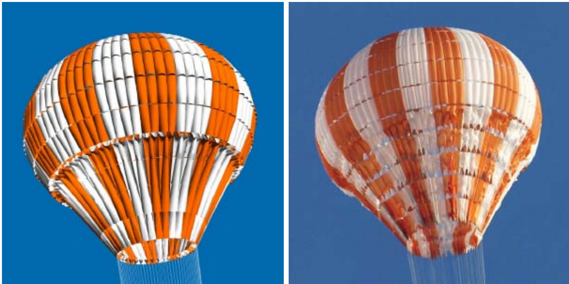
Figure 4: Structural mechanics solution for the parachute reefed to \tau_{REEF} = 13\% (approximately). Left: obtained with the SCFSI M2C computation and the refined structure mesh. Right: picture from a NASA drop test.
