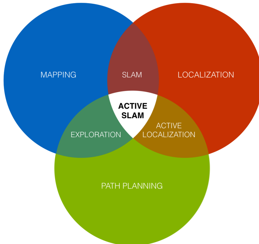
Figure 1.1: Combining the three main problems in mobile robotics, four new problems arise.
