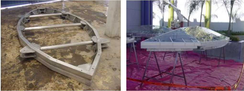
Figure 5: Lantern made with structural steel and tempered glass.
