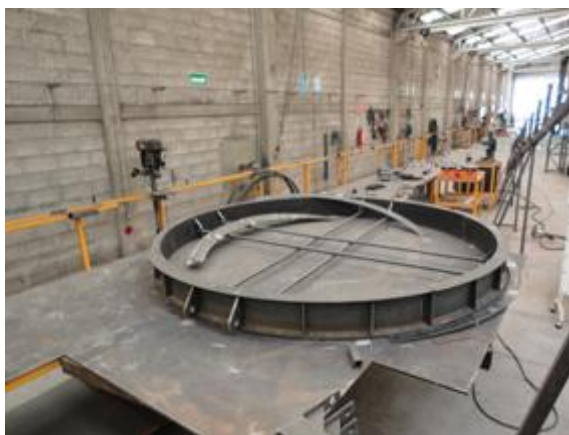
Figure 3: Detail of the lantern and construction of the replacement lantern
