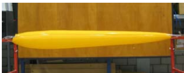
Figure 26: spindle asymmetric tensairity, version 1
