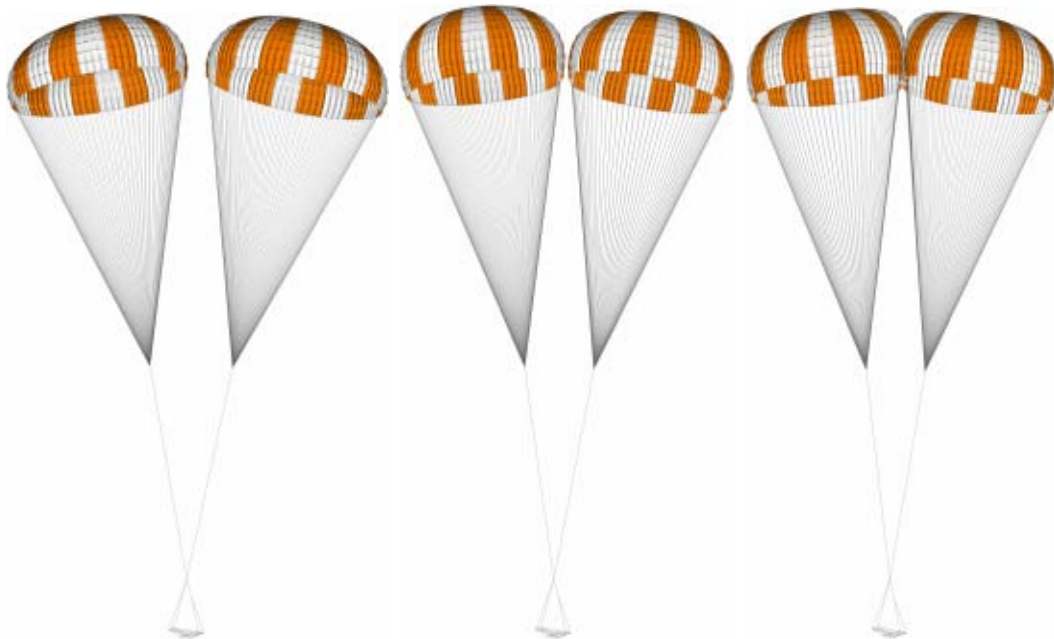
Figure 7: Parachutes at t = 52.20 s, t = 53.36 s and t = 54.52 s during the asynchronous-disreef computation modeling the contact between parachutes.
