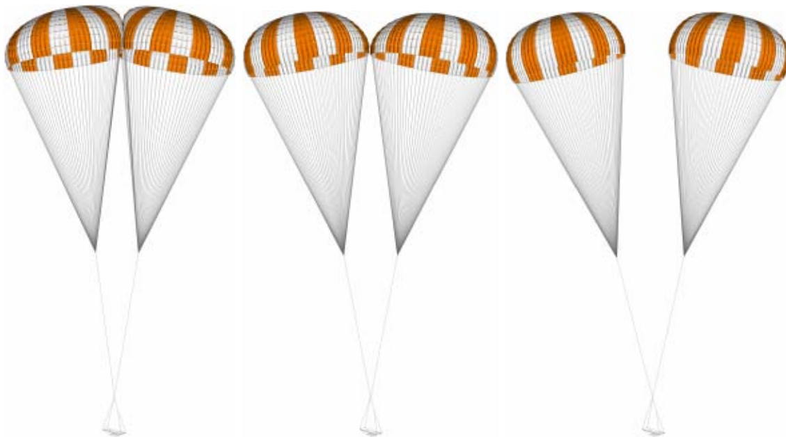
Figure 8: Parachutes at t = 55.68 s, t = 56.84 s and t = 58.00 s during the asynchronous-disreef computation modeling the contact between parachutes.
