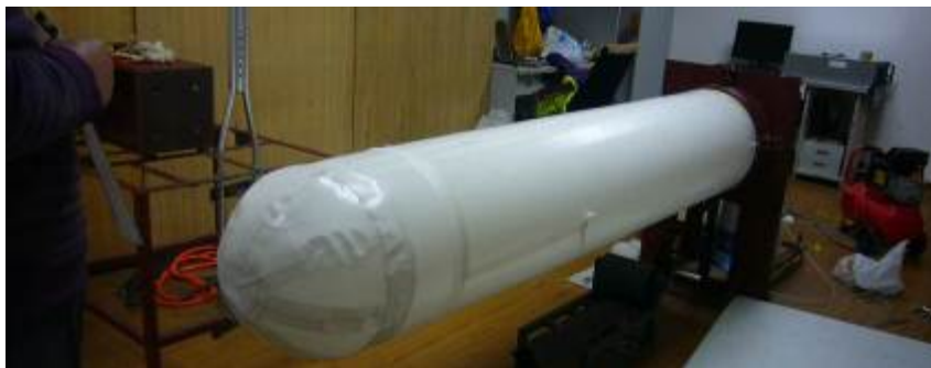
Fig.11: Experiment of the airship envelop inflated beam under bending
