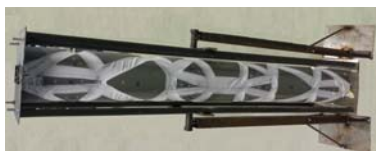
Fig. 15. Mould and falsework for the concrete scale models
