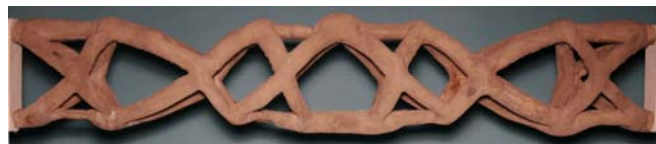
Fig. 15. Mould and falsework for the concrete scale models
