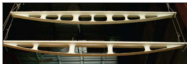
Fig. 6. Optimized beam with fabric formwork 3
