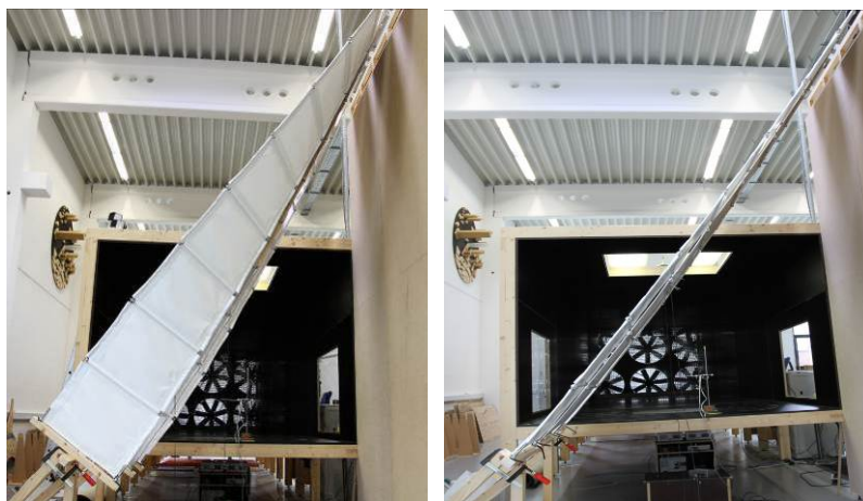
Figure 6: Wind tunnel tests of twisted and planar membrane strips (Wacker Ingenieure - Wind Engineering).
