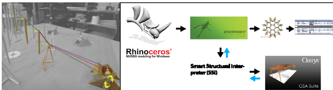
Fig. 18. Movement of the radial tension cables to achieve sliding Fig. 19. Collaboration between the programs 25 26 27 28
