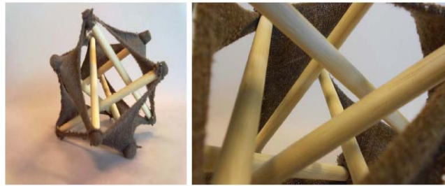
Fig. 8. Tensegrity with membrane
