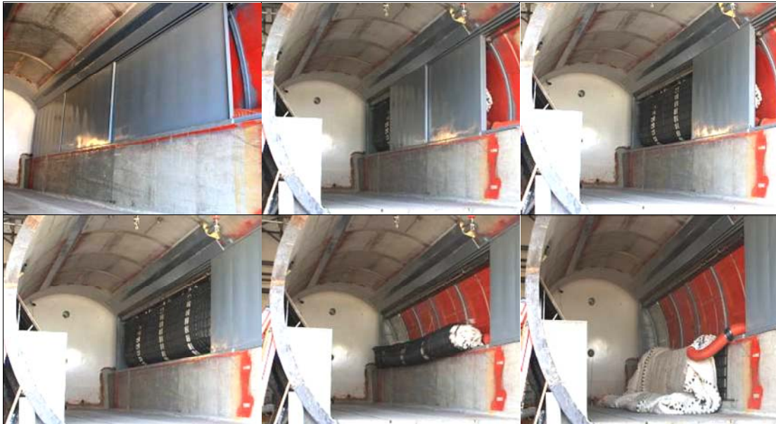
Figure 3: Sequence of container door opening and initial deployment.
