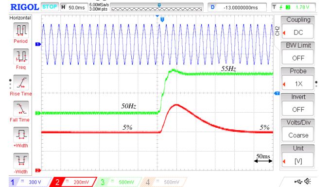
Fig. 22. THD experimental results to frequency step perturbation from 50Hz to 55Hz. The grid has a permanent 5 th harmonic distortion with a 5% amplitude. Ch. 1: Grid voltage (300V/div). Ch. 2: THD (200mV/div or 2.5%/div). Ch. 3: Estimated frequency (500mV/div or 5Hz/div).
