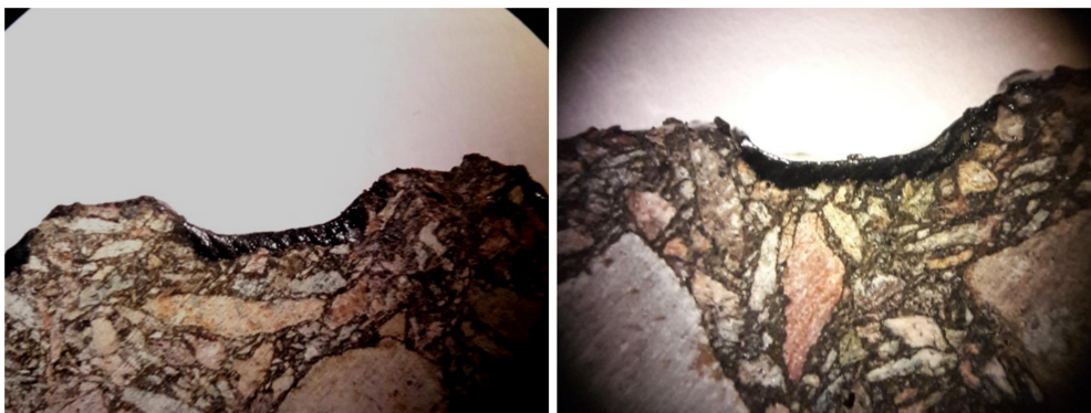
Figure 8. Disposition of tack coat achieved in laboratory.
