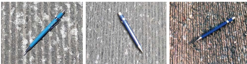
Figure 7. Types of milling (Bonfim 2008).
