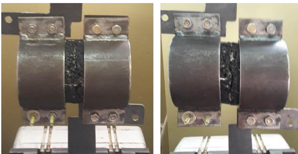
Figure 5. Deformation in the central area of the double specimen during the test.
