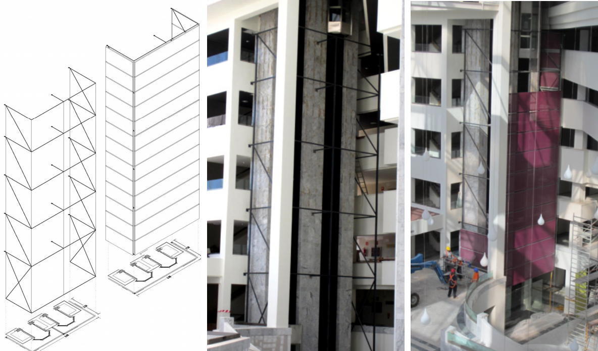
Figure 11: Panoramic elevators: BATenso textile façade framing system and steel structure, 3D view, pictures
