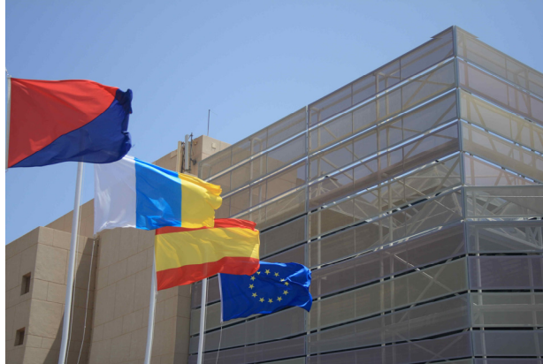
Figure 3: Whilst a flag flutters in a turbulent flow (with high oscillation frequency and fast deformations), a membrane structure gallops in it (low oscillation frequency, slow shape variations).
