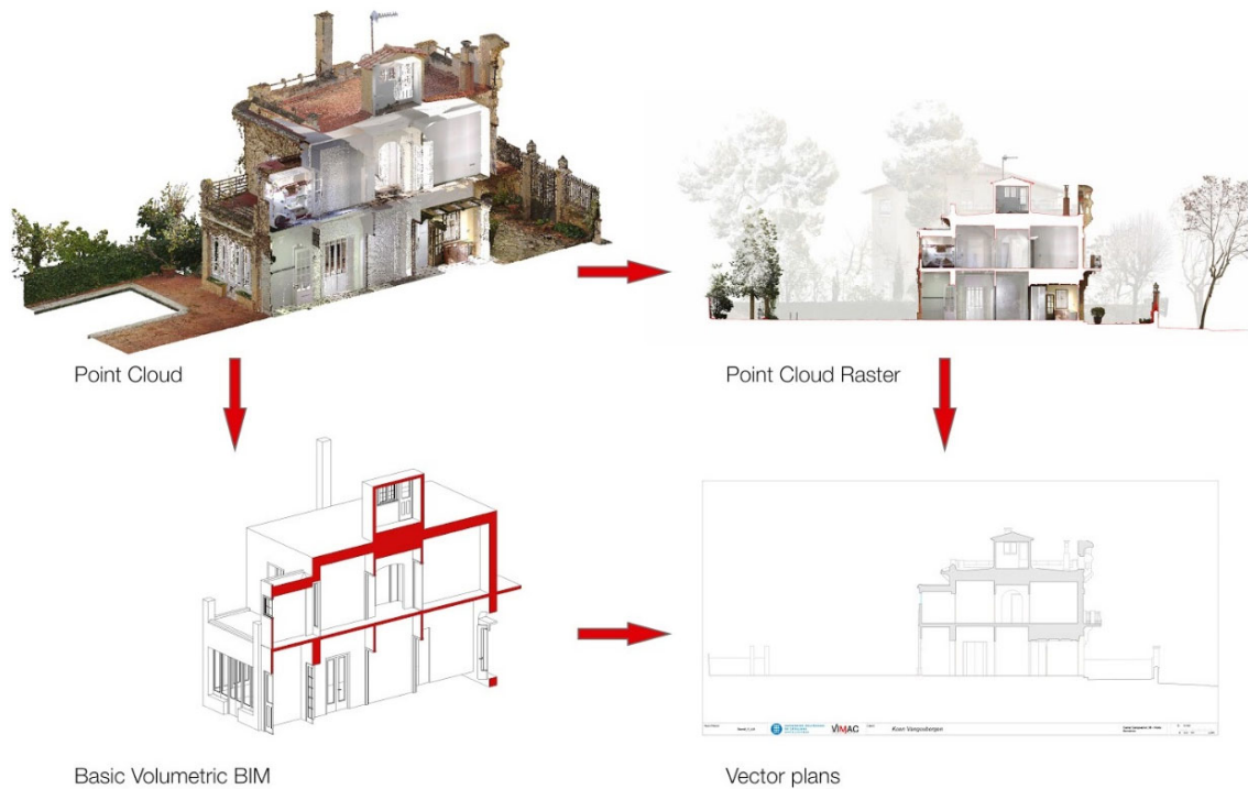
Figure 08. Catalogued house in Barcelona. Diagram of the process to make 2D drawings with Scan to BIM, editing them tracing in CAD with the rasters as a base.
