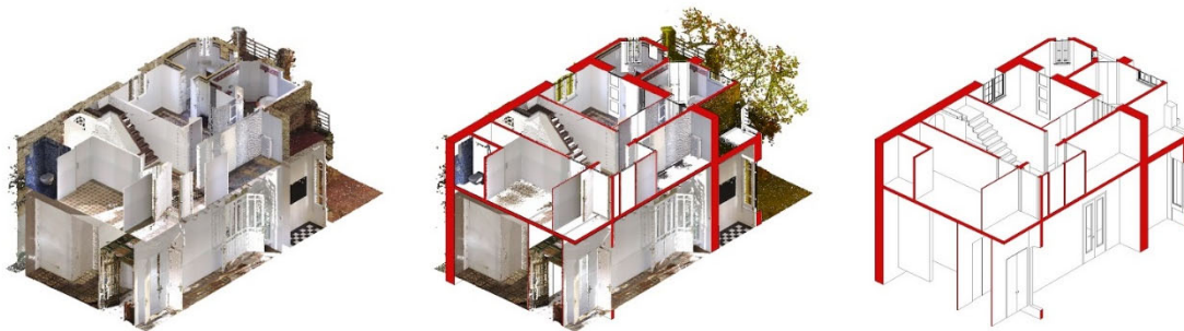
Figure 02. Scan to BIM. From left to right: Point cloud, point cloud with a BIM model overlapped and BIM model.
