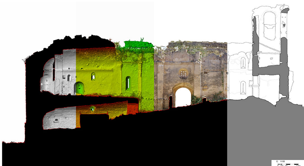
Figure 01. Sant Miquel Montmagastre. Example of a 2D drawing representation: raster 2D with different information and 2D vectorial, from segmentation of a 3D mesh.
