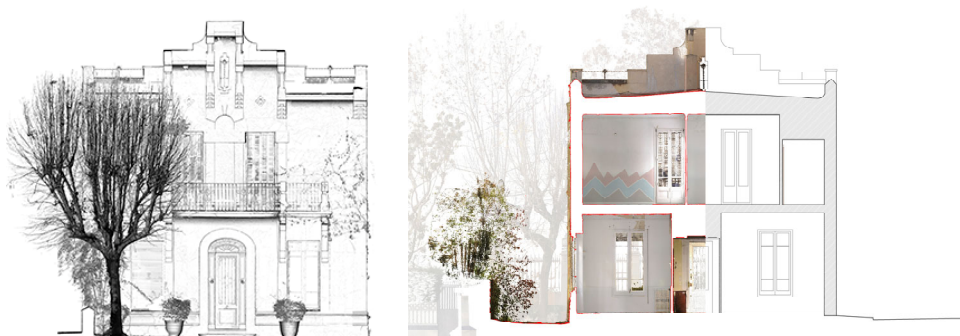
Figure 05. Catalogued house in Barcelona. Raster drawing of the principal façade and a section as raster and vector (CAD)
