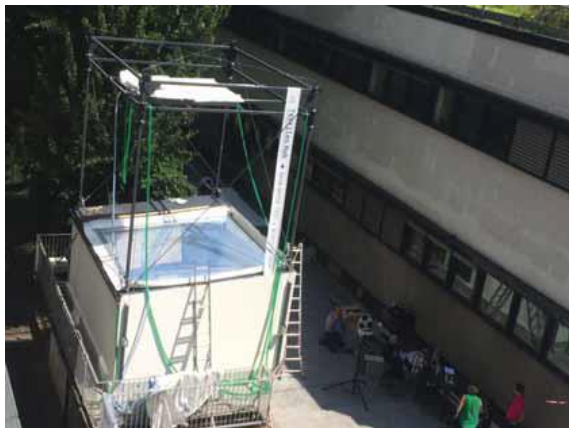
Figure 1 (left): External View of the Test Hut; Figure 2 (right): Detail of the Steel Tank Perforated Base Used for Simulating Intense and Heavy Rain Scenarios.
