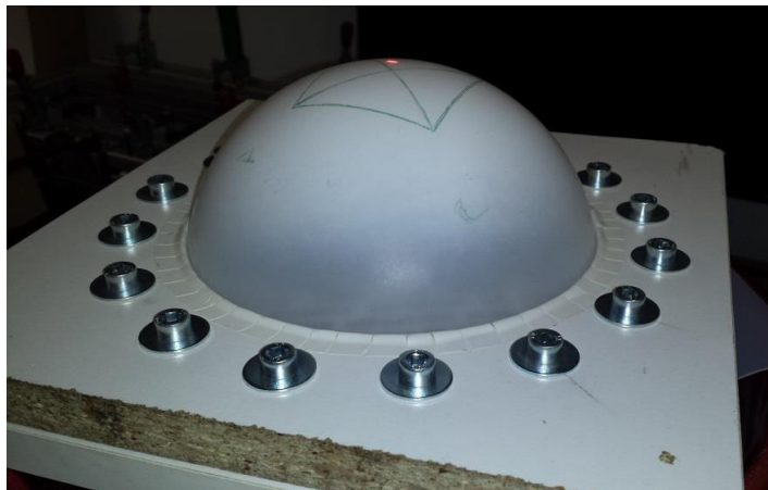
Figure 10: Sample of Wacker R360 inflated to an apex stretching of 86%
