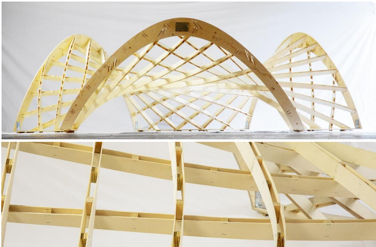
Figure 9: Timber prototype. The lamellas are doubled and coupled to allow for low bending radii and high stiffness. Image: (Eike Schling)
