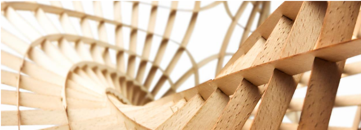
Figure 2: Grid structure based on asymptotic curves: The model is built from straight strips of beech veneer. All joints are orthogonal. Image: (Denis Hitrec)
