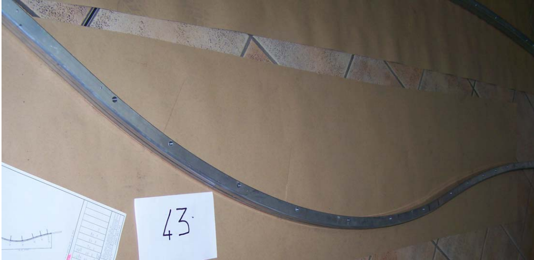
Figure 13: work shop control template
