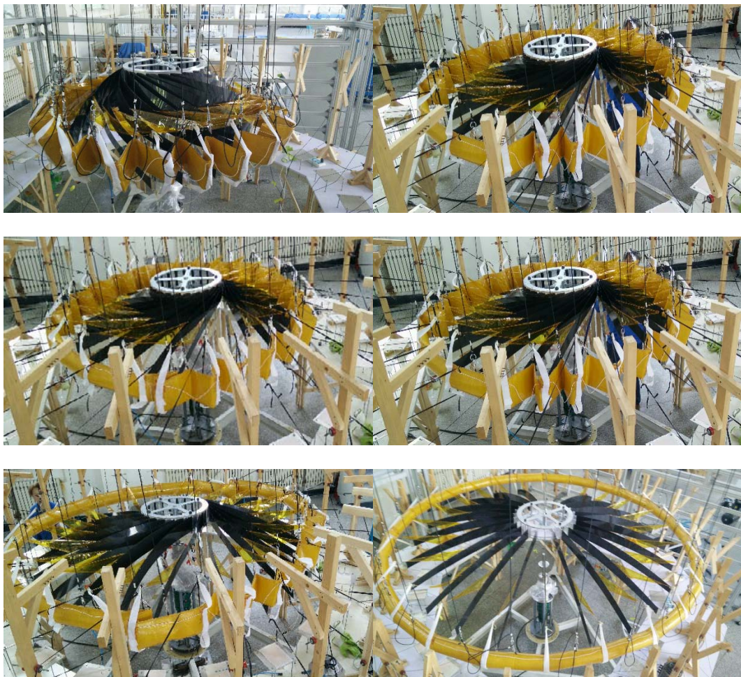
Figure 9 Inner gas pressure driven deploying sub-process
