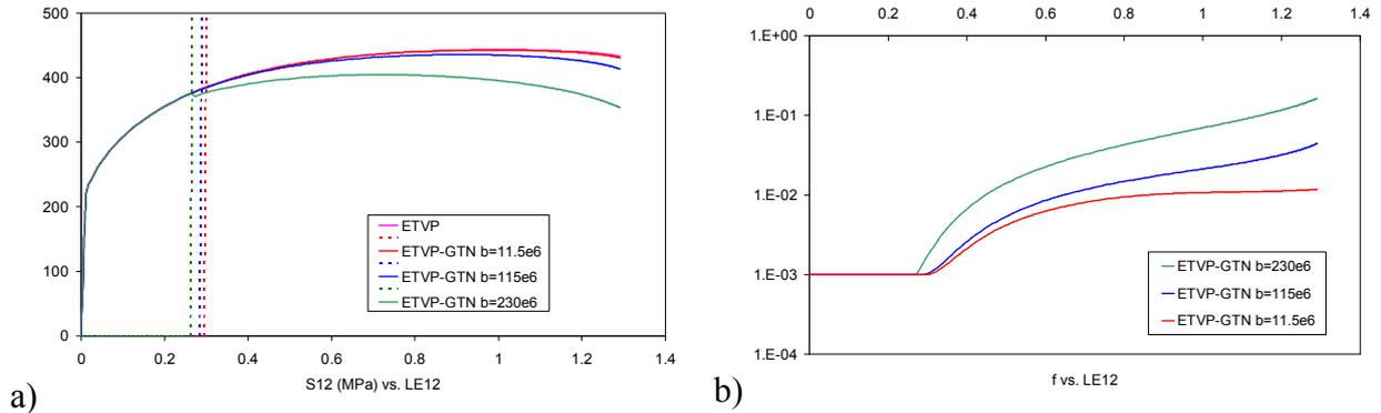
**Figure 4:** Influence of kinematic pressure. Simple shear on a cube.
