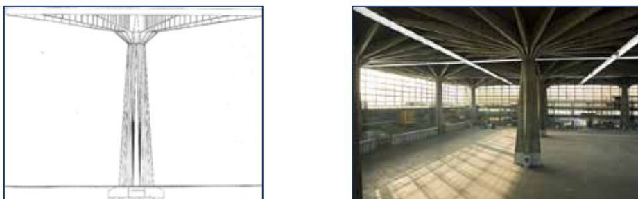
Figure 3: Elevation design drawing and view of a mushroom steel roof panel and the supporting R/C column
