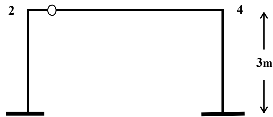
Fig. 5. Schematic representation of main damage in the studied frame subject to Tabas excitation
