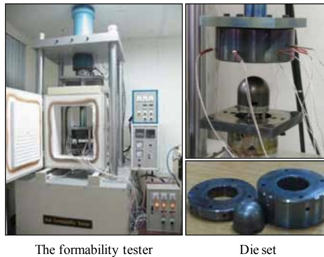
Figure 1: The formability tester and die set
