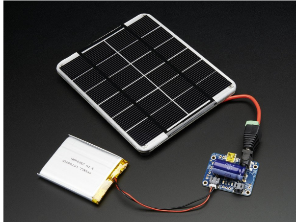
Figure 2.24: Node's independent energy system [94]
