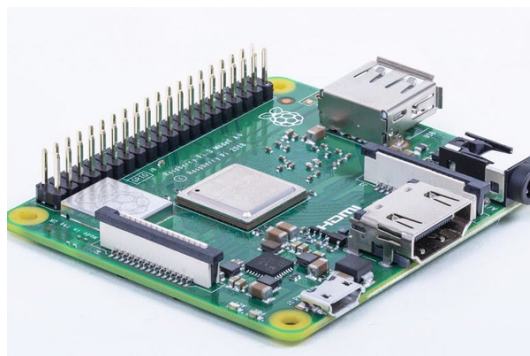
Figure 2.11: The Raspberry-pi embedded platform (Model 3b+) [65]
