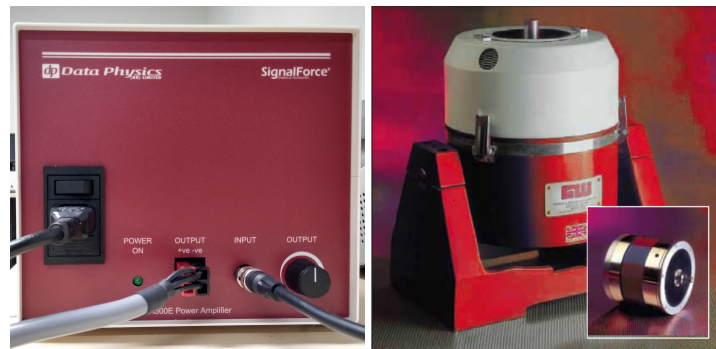
Figure 3. Amplifier model PA300E (left) and inertial shaker IV47 series (right) from Data Physics used in the experimental set-up.
