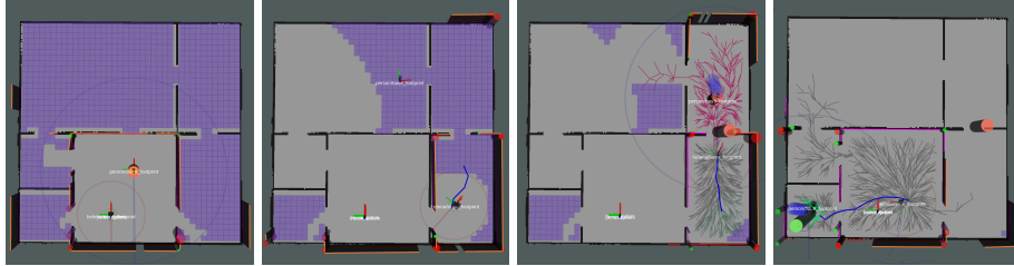
Fig. 2. Collaborative Search Testbed. From left to right: a) The robot infers the unexplored zone from its detection range (red circle) and the person’s (blue circle). b) People detection is impossible when the person is out of sight, hence no inference is done. c) The person indicates the robot to avoid searching through that zone, as either it is already explored or the person will do it on their own. d) The person finds the object, thus indicates the robot to come.
