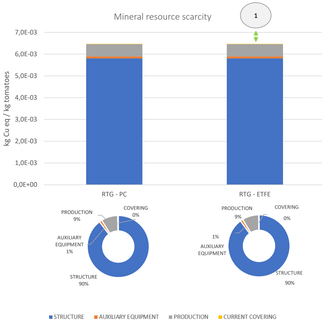
Figure 29. Comparison, based on Mineral resource scarcity, between the current RTG with polycarbonate covering and the optimised version: RTG with ETFE cover.
