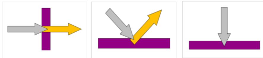
Figure 3. From right to left: transmissivity, reflectivity, absorptivity.
