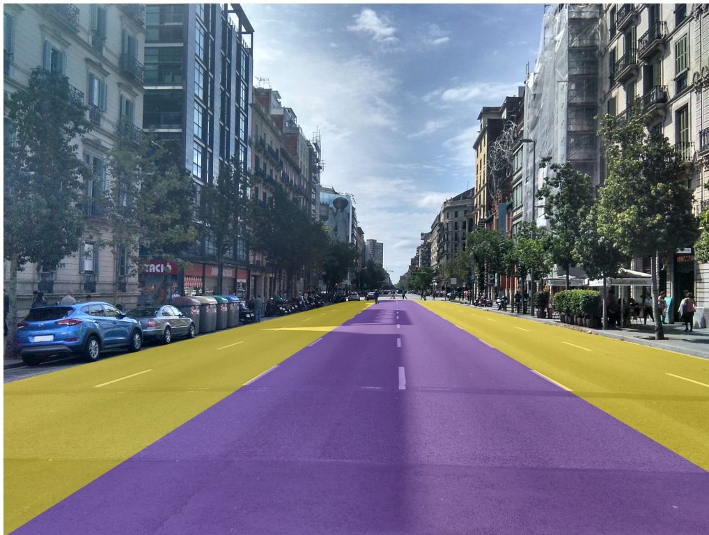
Figure 40: Rendering of the double CAV-ONLY lane considered for Scenario B . Lanes in yellow are destined to mixed traffic flow, but the central lanes (violet) are reserved as CAV-ONLY lanes. OWN ELABORATION.
