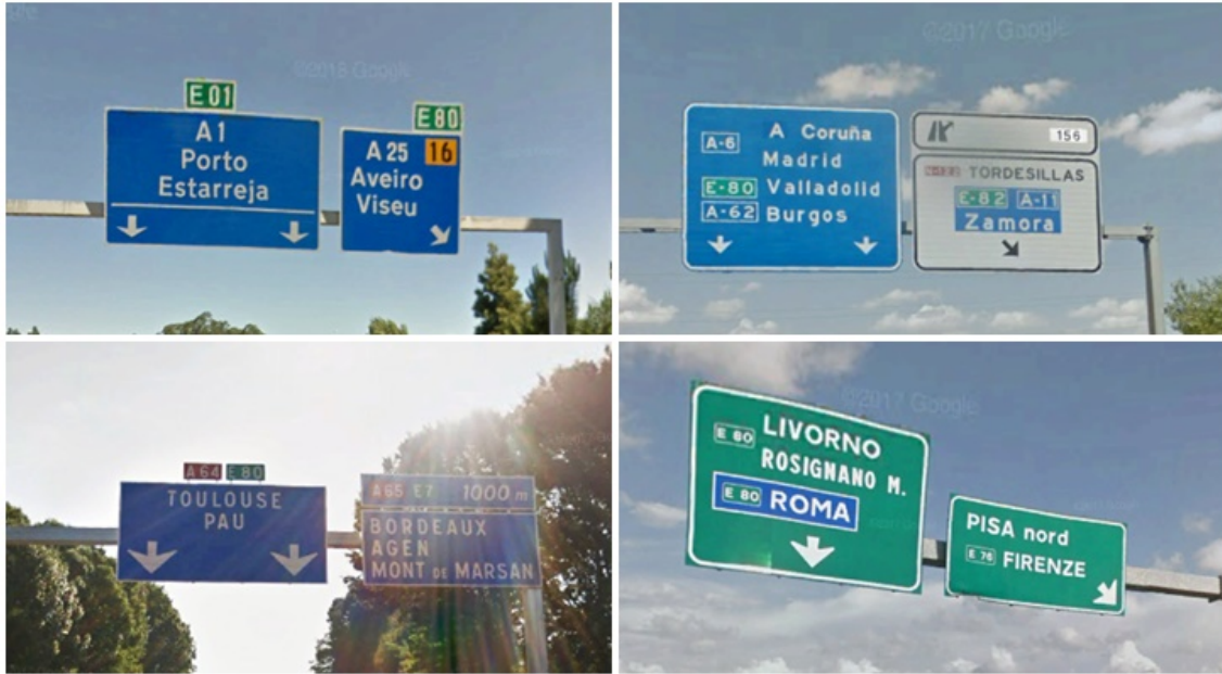
Figure 6: Indication signage variations between some European countries: Portugal (top-left), Spain (top-right), France (bottom-left) and Italy (bottom-right). Notice that each sign corresponds to a junction where E-80 European route meets other major European routes. GOOGLE MAPS.
