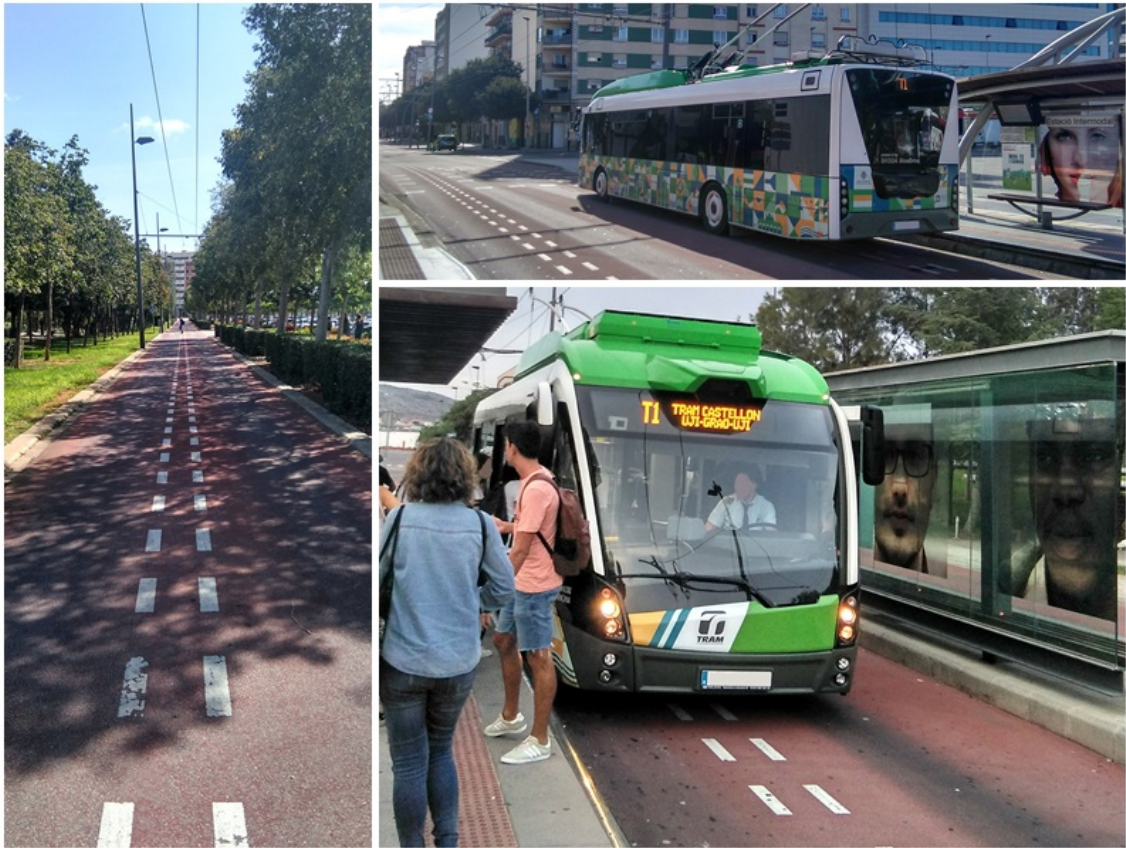
Figure 36: Semi-autonomous trolleybus that links Castellon Harbour (Grao) with Jaume I University Campus (UJI) in Castellon, Spain. Notice that the dedicated lane for such service is equipped with two parallel sets of markings which create a fictitious track which is being observed by a computer-vision camera placed over the info panel of the trolleybus. OWN ELABORATION.
