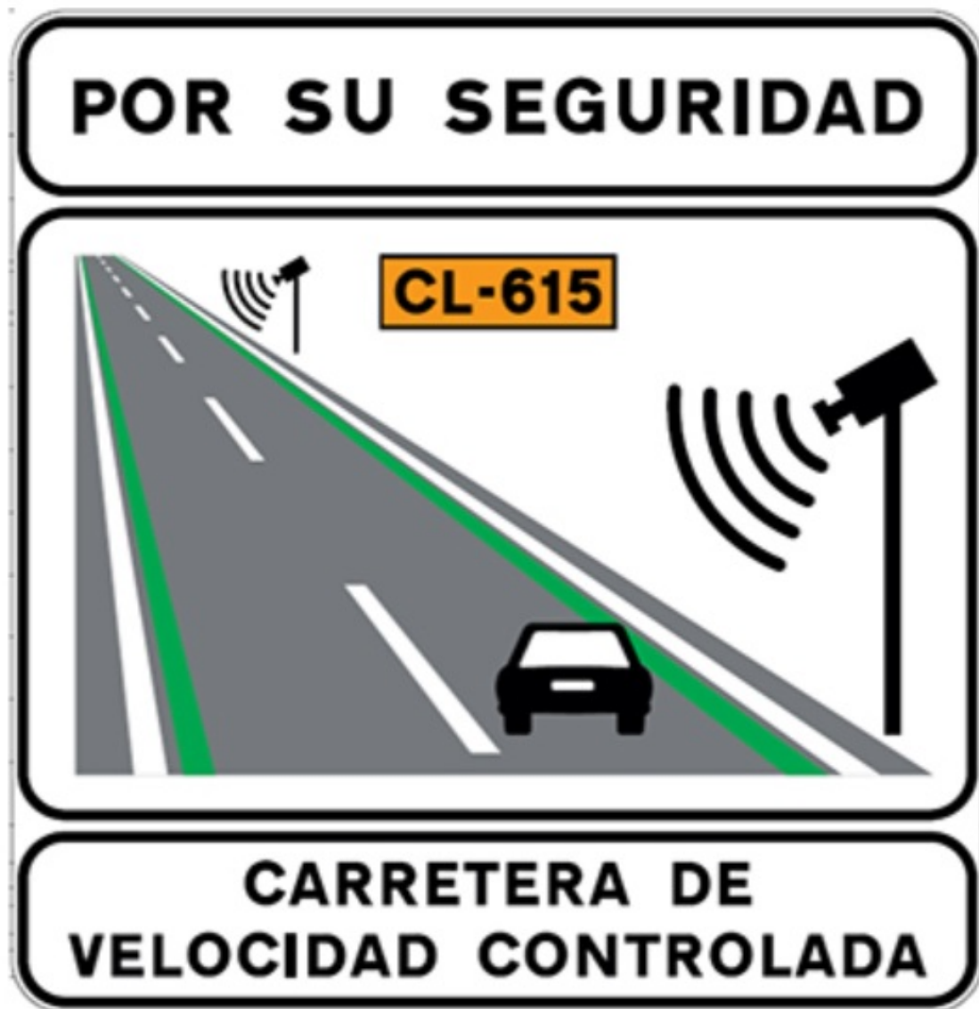
Figure 3: Spanish sign which indicates that green marks on asphalt mean that a speed control may be being carried out.
