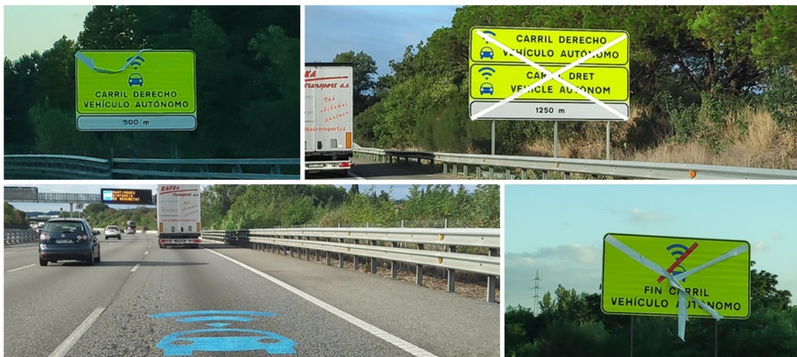
Figure 34: Newer traffic signs in Girona, Spain that inform about the existence of a CAV-ONLY lane destined to the performance of the testings related to project INFRAMIX. TWITTER (@punsix)
