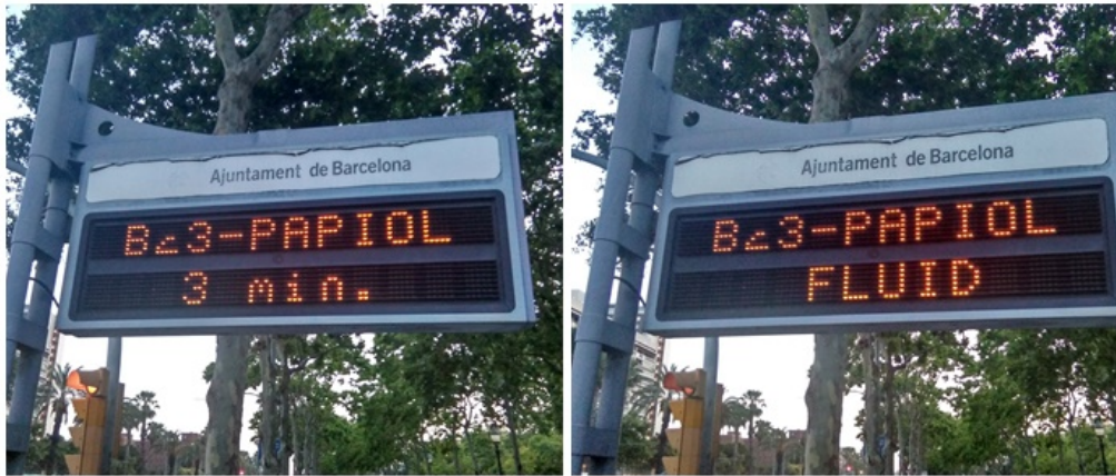
Figure 18: A variable message signage panel in Barcelona which is showing some information about the current traffic state and the expected time that a vehicle will spend on reaching the next highway section. OWN ELABORATION.
