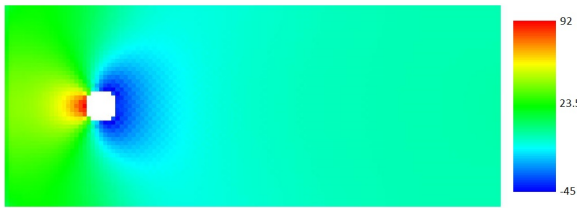
Figure 88: Pressure field at Re = 10
