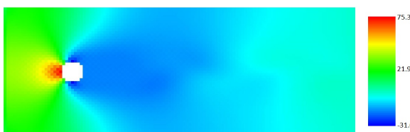
Figure 94: Pressure field at Re = 2000
