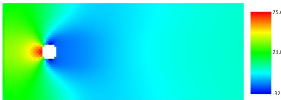
Figure 90: Pressure field at Re = 100
