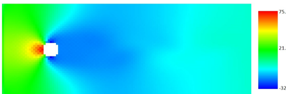
Figure 92: Pressure field at Re = 500
