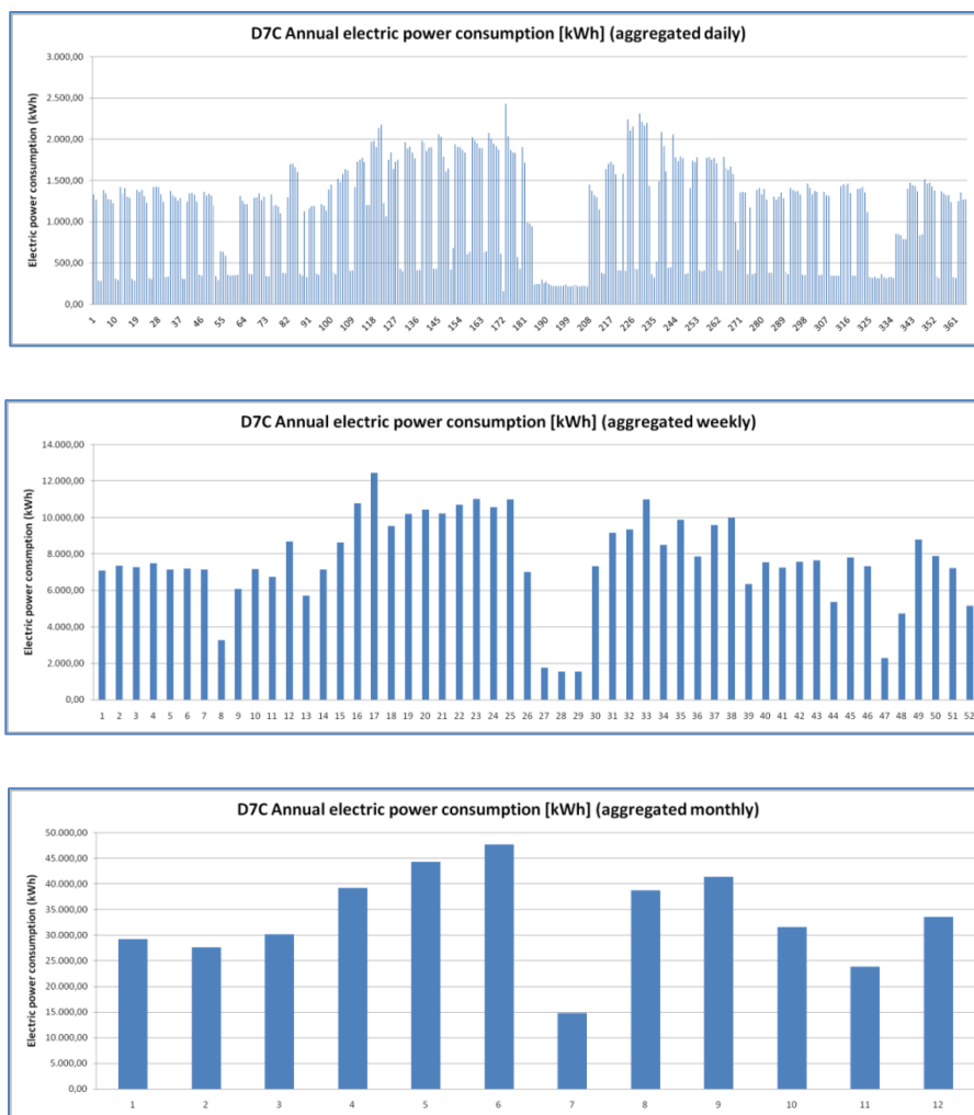
Figure 41. Electricity consumption for D7C Building: daily, weekly and monthly basis. Source: SIRENA and own elaboration.
