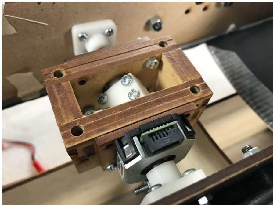
Figure 5.4: Close view of assembled gimbal
