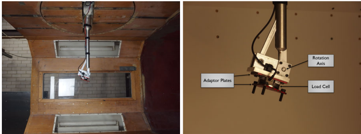
(a) 3x4 mount in wind tunnel test section (b) Close-up of mount rotation mechanism and load cell
