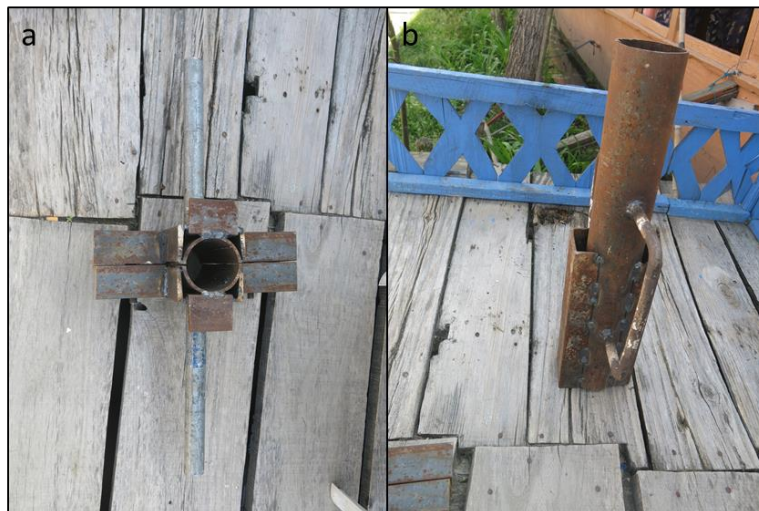
Figure 4.2: a) Striking platform; b) slide hammer used in percussion coring.
