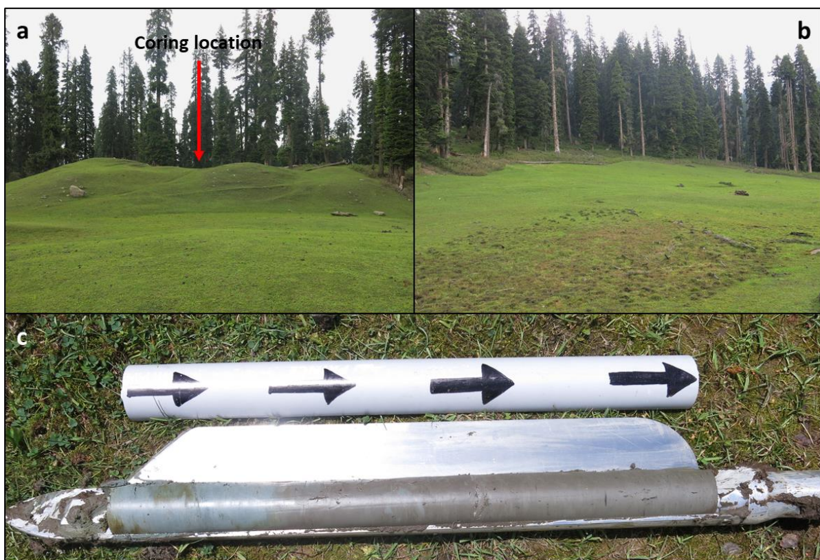
Figure 4.9: SG02: a) hummocks around mire; b) sampling site; c) blue-grey unoxidised clay at lowest sample depths.
