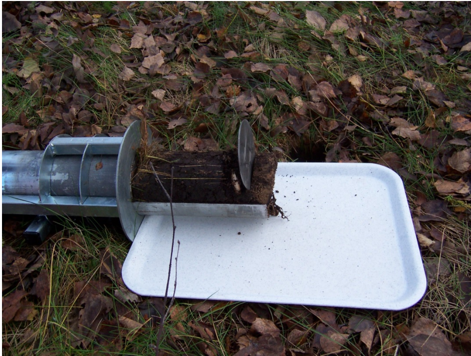
Figure 1. Slicing of a soil sample taken with a golf hole cutter. Photo: STUK.
