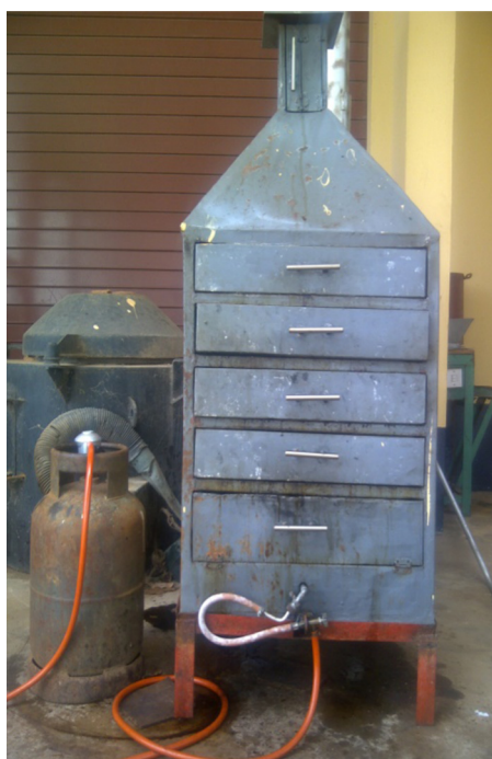
Fig. 2. Pictorial view of the gas-fired cabinet dryer.
